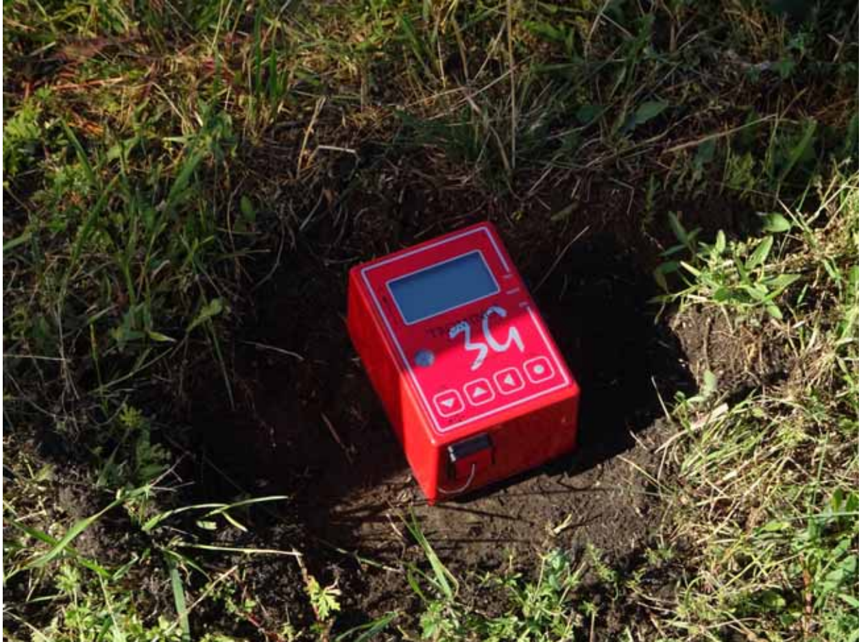
Pic.7 Seismograph Tromino 3G, Seismic noise measurement.
