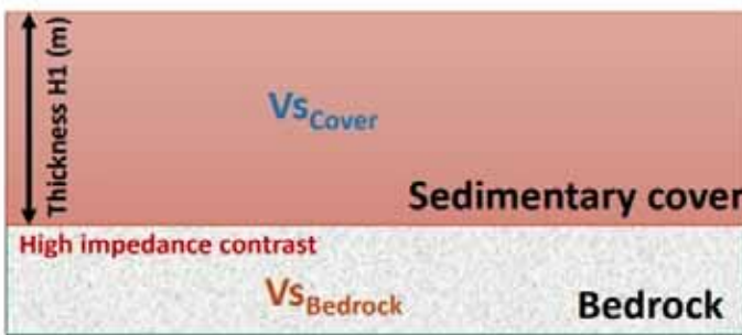
Pic.5 The basic case with one main subsoil Resonance frequency
