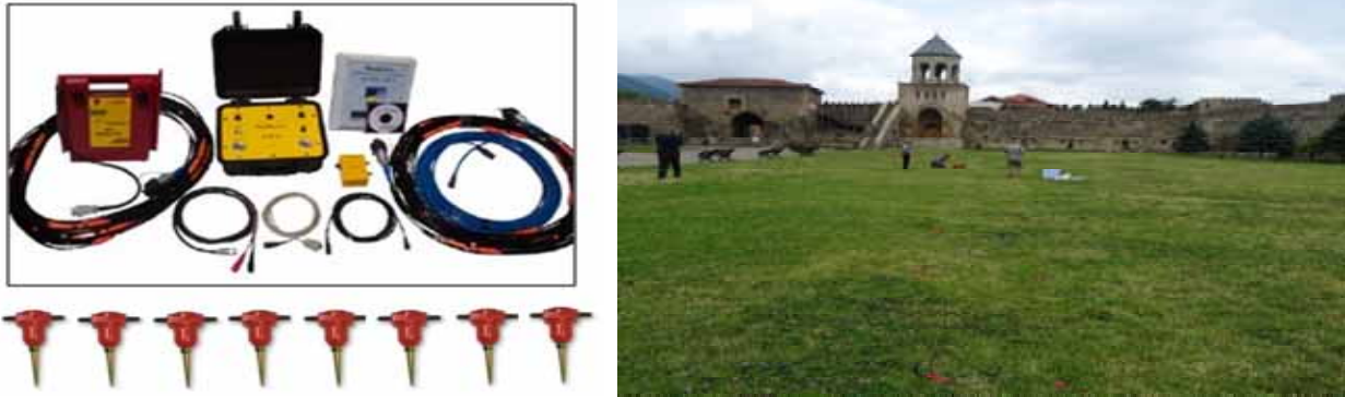
Pic.2 seismic refraction tests with RAS-24 multi-channel survey, for using 4.5 Hz vertical geophones.
