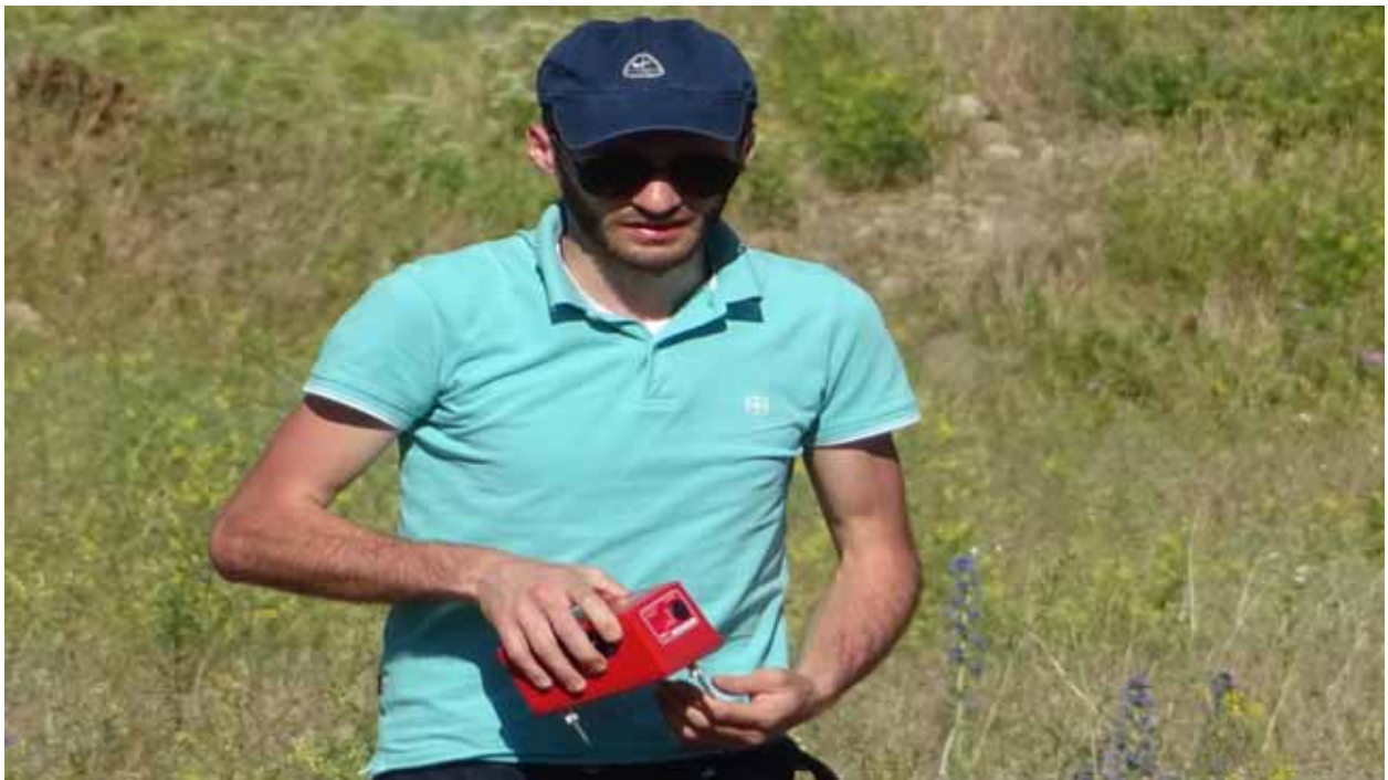
Pic.7 Seismograph Tromino 3G, Seismic noise measurement.
